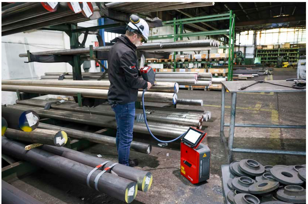
SPECTRO Analytical Instruments has introduced the SPECTROPORT LIBS PXL01 portable OES metals analyser for metals analysis in the field
